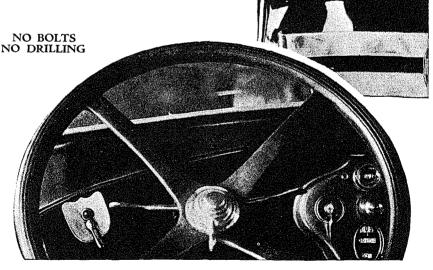
Control Right at the Wheel Switch Completely Wired With Tell-Tale Light
