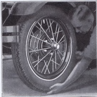
Figure 26 Centering Tire on Rim
