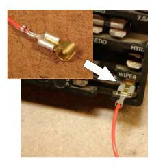
Connect the RED wire of the red/black wire pair to the fuse panel (if equipped) to a KEY-ON-HOT connection. Use either of the enclosed brass fuse adapters if your fuse panel lacks an accessory tab.
