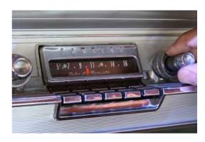
4. Turn the radio on and tune to 1000 kHz on the AM band.
