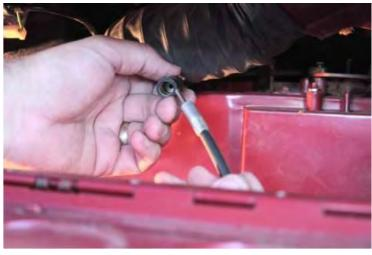
Plug the vehicle's antenna cable into the RediRad™ antenna cable jack.
