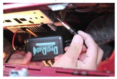
Insert the RediRad™ male plug into the radio's antenna cable socket.
