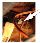
Connect the BLACK wire of the red/black wire pair to vehicle GROUND as shown.
