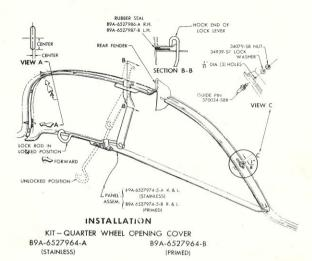
Before color painting Panel Assembly, three  $\sqrt[8]{2}$ " dia. holes must be drilled in Fende: Flange for attaching Guide Pins. (See View C).
