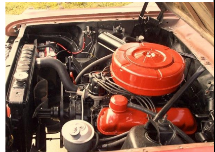
The above examples are a 260 Cyclone V8. You can clearly see the special Orange/Red color scheme. Also the snorkel and heat collector can be seen in semi gloss black. Oil filler cap should be semi gloss black also.
