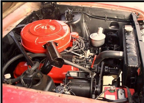
The above examples are a 260 Cyclone V8. You can clearly see the special Orange/Red color scheme. Also the snorkel and heat collector can be seen in semi gloss black. Oil filler cap should be semi gloss black also.
