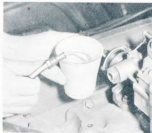
Checking Fuel Flow
