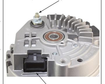
When using with OEM wiring harness, plug in factory connector here
